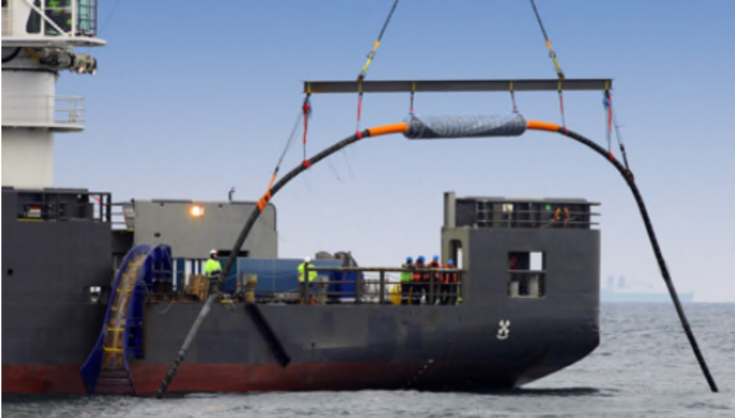
Figure 10.3-12: Vessel lowering an offshore cable joint using a bow.
