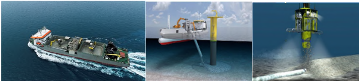
Figure 10.3-8: Typical images of Rock Dumping Vessel, Fallpipe, and ROV controlled lower end.
