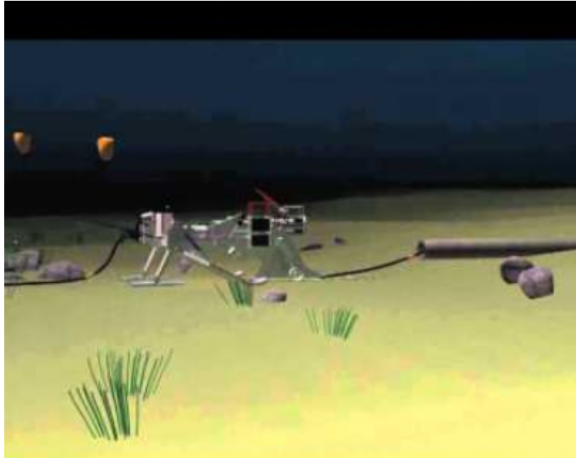
Figure 10.3-11: Indicative picture of a plow burying a cable.
